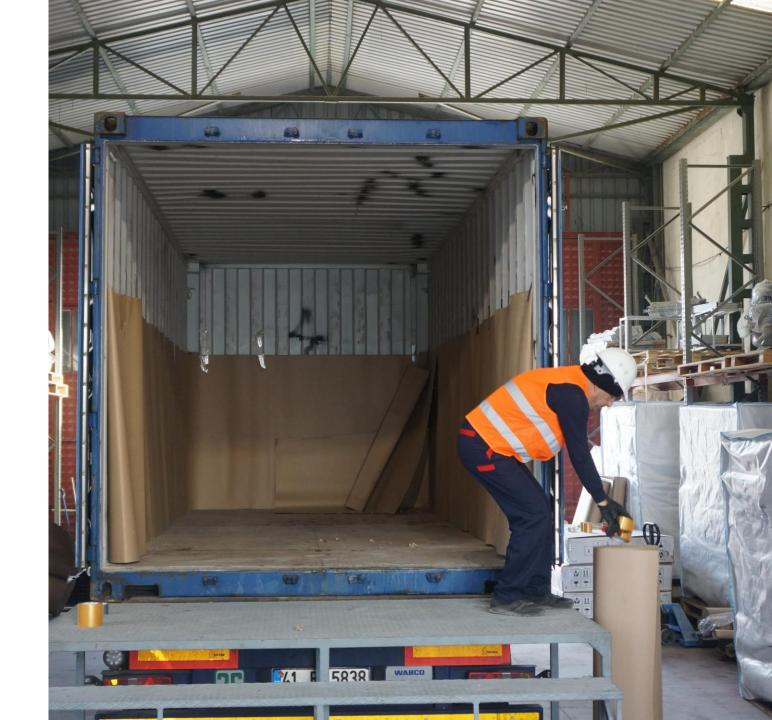
The Flexitank is opened within the container from back to front and laid out on the ground whilst keeping the filling valve on the right side. The container is not entered with shoes during laying out.
