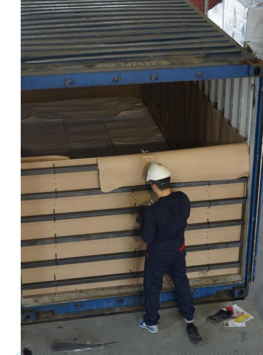
A vertical support bar is added towards the right side of the left container door. The left door is closed. This way, pressure to the container door during carriage is reduced.
